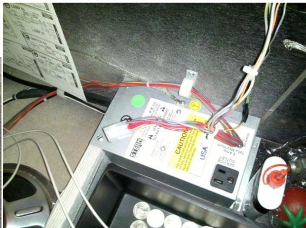
Step 4: Plug your existing backbox panel into the female plug with the shorter set of wires coming off of the dimmer module.
