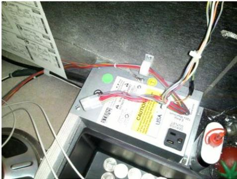
Step 2: Plug the two pin connector into the Dual Relay Board.
