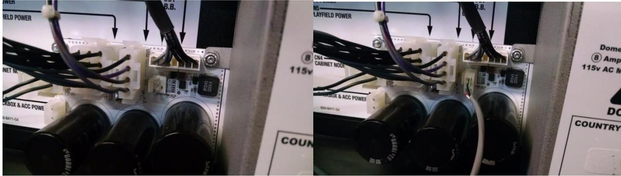
Step 2: Plug the two pin connector into the Relay Board.
