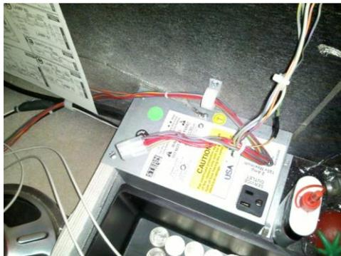
Step 2: Plug the two pin connector into the Relay Board.
