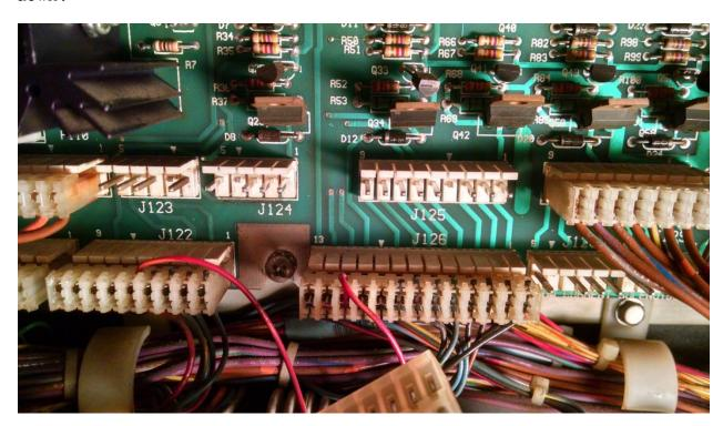
Now plug the female connectors of the purple board to the male plugs on the games board, it may be hard to push on, that's normal. Then plug the games female plugs down onto the purple board. The connectors should be keyed to only plug into the correct places. Depending on your game it may be easier to
