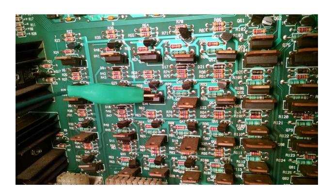
Step 7: The next step is to connect the little 4 pin connector board to the game. Locate J116, J117 and J118 in the lower left of the same power board. This little connector board will plug into any of those. Pick whichever one seems easiest to you, especially if one isn't used in your game. Use the same process with this board, unplug the connector, plug the kits connector onto the board then plug the games connector onto the kit.
