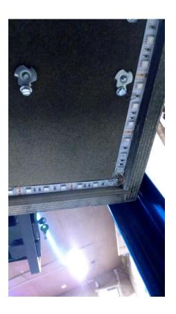
Step 9: Plug the LEDs four pin connector into the kits four pin connector you put through the grate earlier then tuck any extra wire back up into the game. That should be it for the installation! Put the game back together, checking to be sure no electrical components from the game touch the Smart Board, and turn it on!
