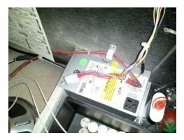
Step 2: Plug the two-pin connector into the Dual Relay Board.
