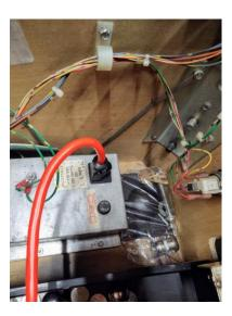
Step 2: Mount the power supply in an out of the way place by pealing the adhesive strips off of the back of it and pressing it in place.
