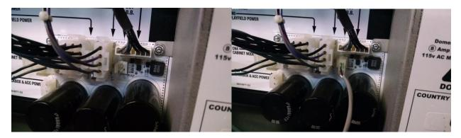
Step 2: Plug the two-pin connector into the Dual Relay Board.
